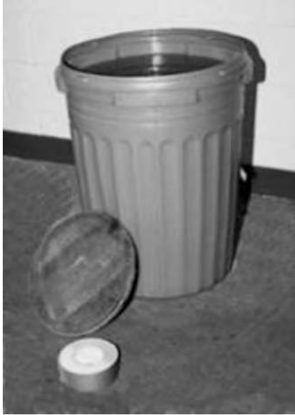
FIGURE 9.1 Plastic explosive container (PEC) with steel plate that gets seated inside the bottom of the container.
