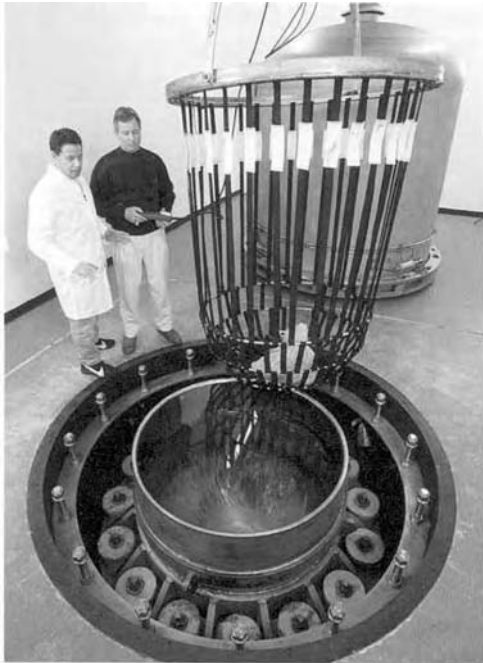
FIGURE 9.2 Stationary 1060-L commercial prototype steel vessel (CHU) with 16 shock absorbers.
