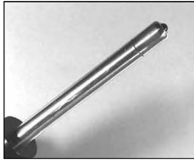
FIGURE 5.12 Immersion ball probe for robust Raman measurements.
