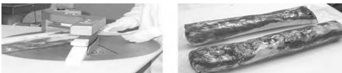
FIGURE 4.3 Sealing Pi-Vac film after insertion and loins that have been Pi-Vac packaged.
