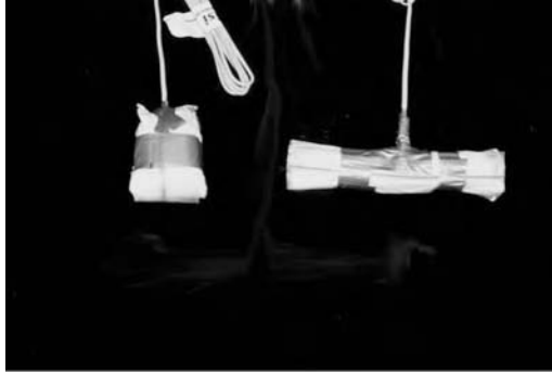
FIGURE 9.6 Shape of charges: Charge on left is rectangular (folded) shape; charge on right is cylindrical shape.
