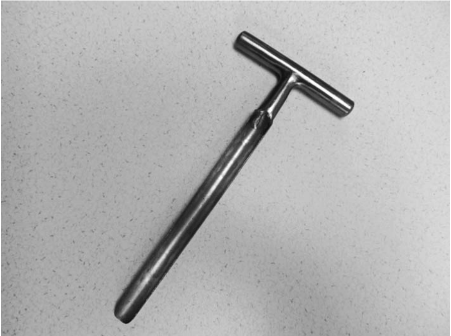
FIGURE 3.2 A trier is pushed or twisted into a block of cheese to extract a sample. Source: Author's collection.
