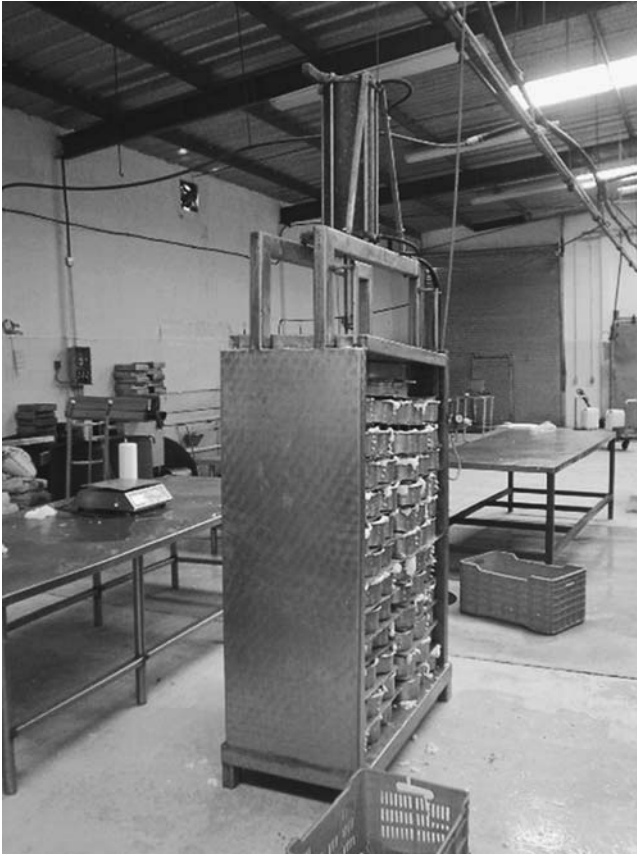
FIGURE 2.10 Vertical cheese press in use. This type of press has a small footprint but creates more pressure at the bottom than at the top.
