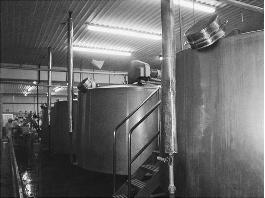
FIGURE 2.2 Elevated double-walled cheese vats. The disk-shaped objects atop the vats cover the stirring motors. Heating/cooling water flows from the vertical pipes into the space between the walls. Source: Author's collection.
