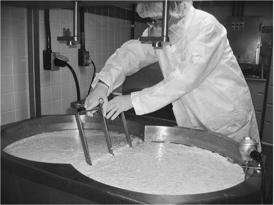
FIGURE 2.5 The author using cheese knives to cut curd.
